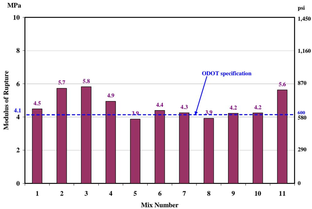
(b) Modulus of rupture at 7 days
