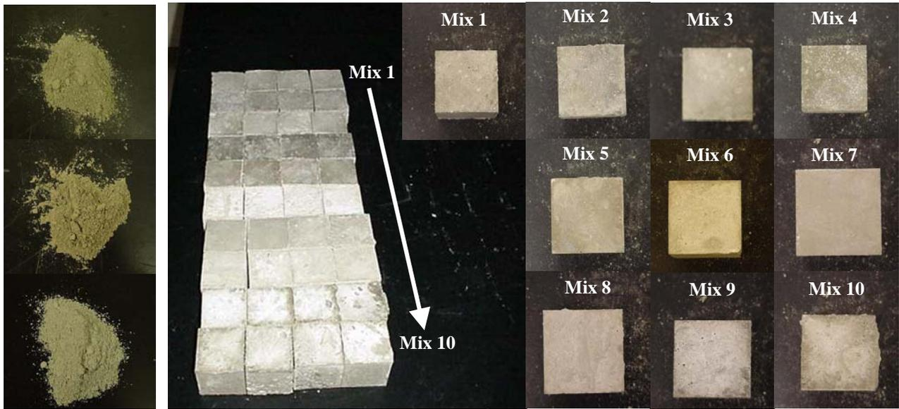
**FIGURE 1 (Left) from top to bottom: cement, fly ash, and slag, respectively; (Right) cube samples for albedo testing**
