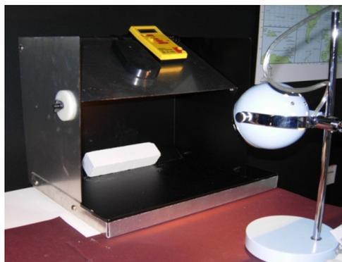
**Figure 4** - Test apparatus for demonstrating light reflection
