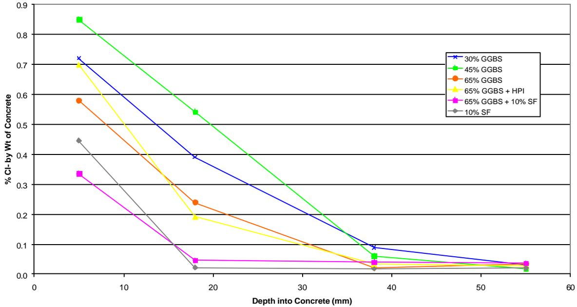
Figure 3: Chloride Penetration into Berth 8 Beams after 19 years
