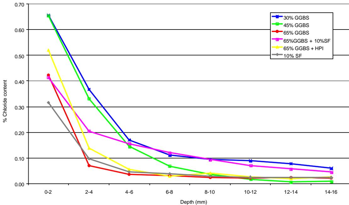
Figure 4: Accelerated chloride penetration into uncontaminated concrete core
