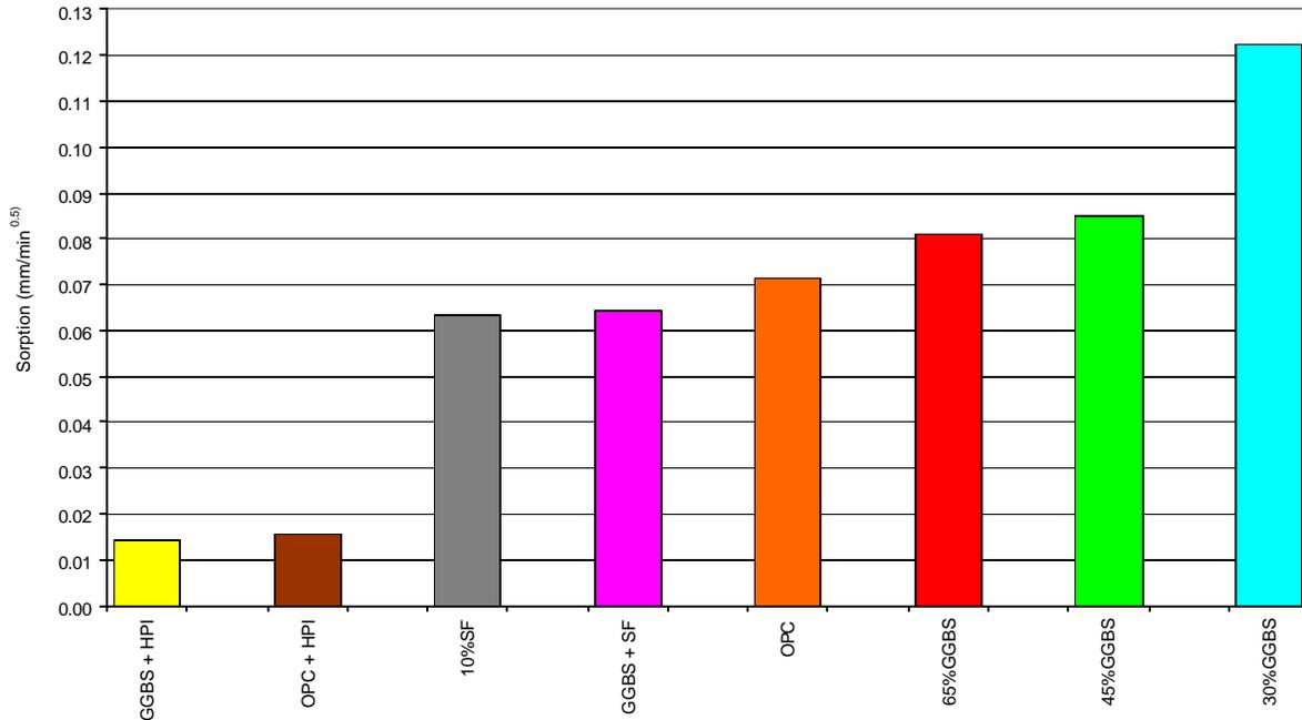
Figure 2: Sorptivity results from concrete after 19 years field exposure.
