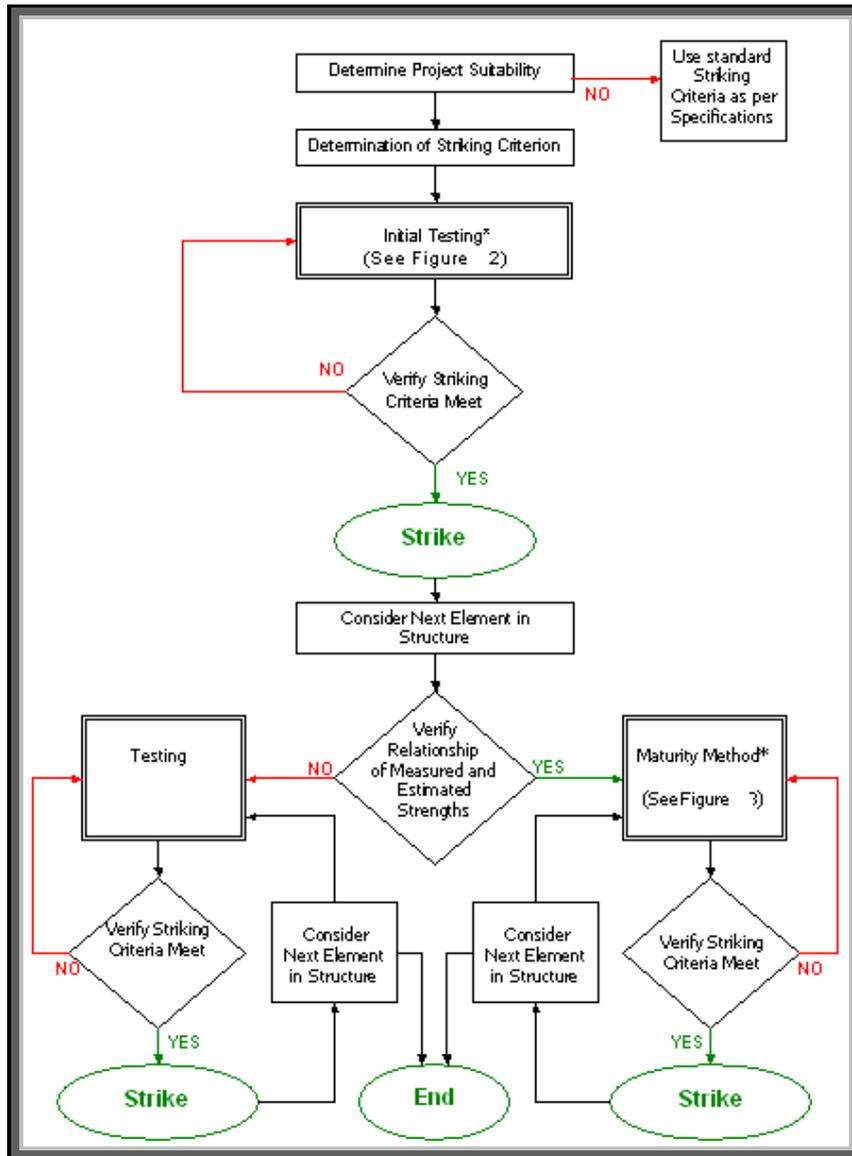
**Figure 1 – Decision-Making Flowchart for the Striking of Formwork**
