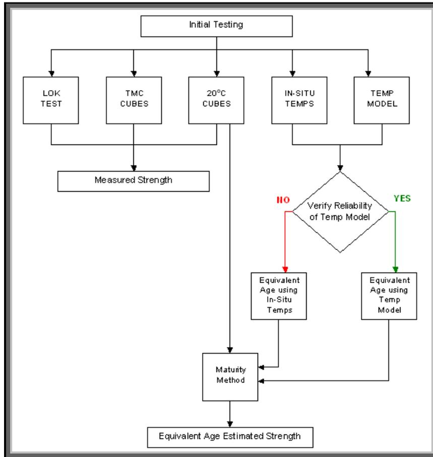
**Figure 2 – Initial Testing Programme, Sub Chart of Figure 1**
