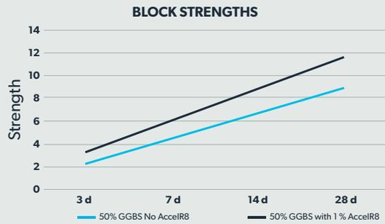
Figure 2 illustrates the strength gains over time by contrasting GGBS with no accelerate and GGBS with 1% AcceIR8 added to the mix.
